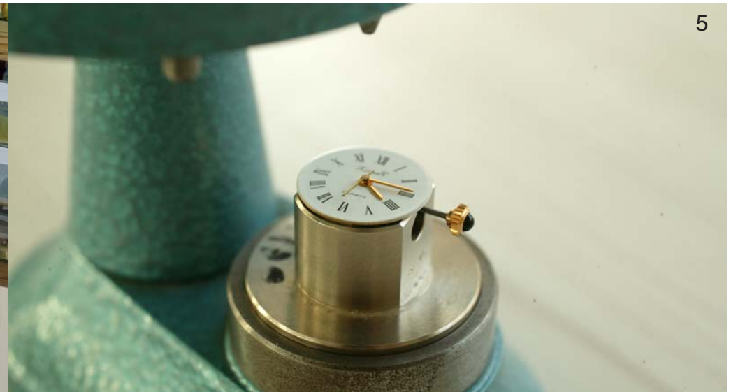
Hands Placement: Nothing in a watch is glued in place. The dial is mounted on the movement using two side screws. Then the hour, minute, and second hands are carefully installed on the dial face at a precise height.
