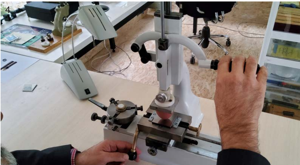
Dial Making is performed by Roger Fermer Precision tampon machine. The ink is first applied to a template, and the transferred to print onto the dial. This procedure requires mastery of the art to use proper concentration of ink, and a retarding agent.
